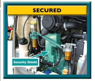
Kosran Secured. The ECV® immobilises the fuel supply, hydraulics & electrics. It is impossible for thieves to hot-wire and electrically bypass the Kosran ECV®
