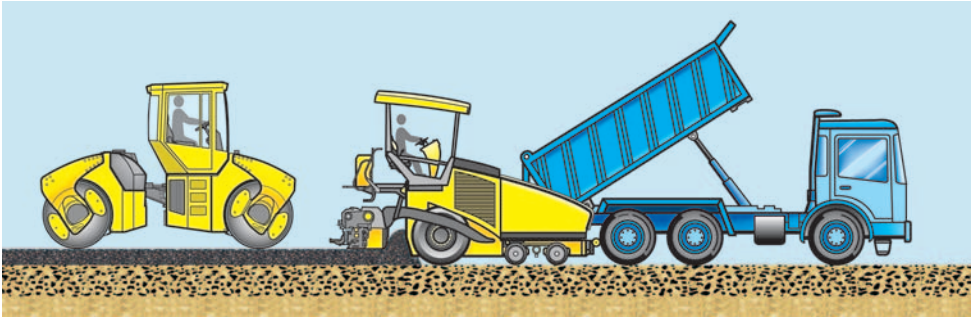
Fig. 6 Initial compaction by the finisher
