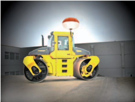
Fig. 43 Tandem roller with 230 V electrical connection
