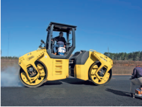
Fig. 42 Articulated roller with ROPS/FOPS
