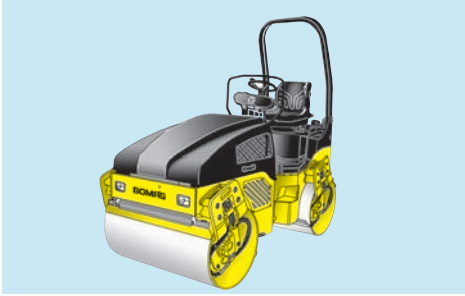
Fig. 17 light, articulated tandem rollers
