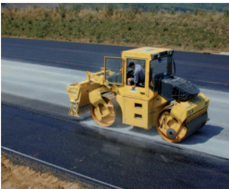
Fig. 72 Chip hopper laterally displaceable
