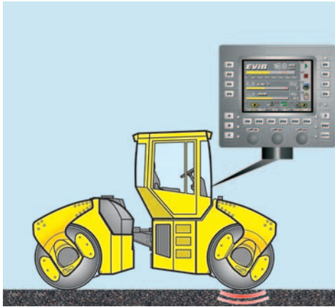
Fig. 82 Asphalt Manager with compaction measuring system
