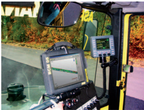
Fig. 87 Continuous compaction control on asphalt CCCA
