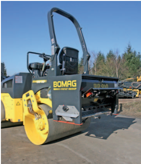
Fig. 41 BW 120 with attachment spreader BS 100 and foldable roll over protection structure
