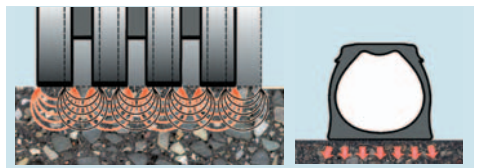
Fig. 56 Pressure distribution and optimal tire contact area
