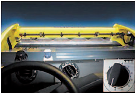
Fig. 29 The sprinkling system
